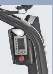
The dashboard in the driver's cab is placed overhead and can be seen when the driver turns his head, and the functions can be pressed easily.
