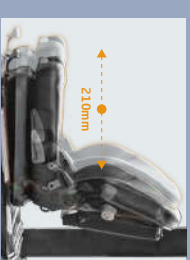
The seat can be adjusted back and forth by 210mm. The operator can choose the best driving position.
